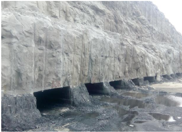
Fig.2. High Wall Mining at West Bokaro, TSL
