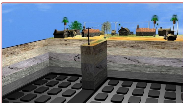
Fig. 4 Conventional Bord and Pillar workings and Subsidence after Extraction
