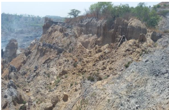
Fig 3 Bench Failure at Manikpur Opencast Mine of M/s. SECL
