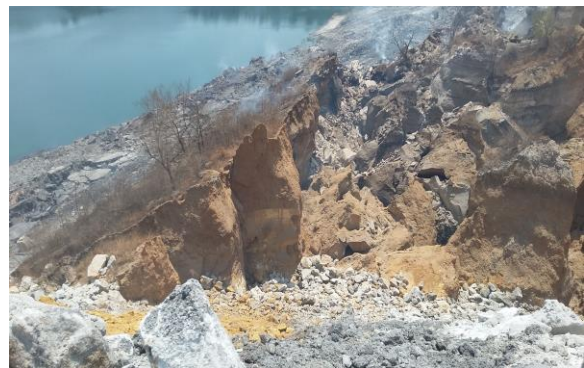
Fig 3 Bench Failure at Manikpur Opencast Mine of M/s. SECL
